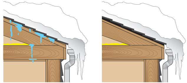
When snow and ice melt, trapped water can infiltrate to damage the roof deck and building interior.
